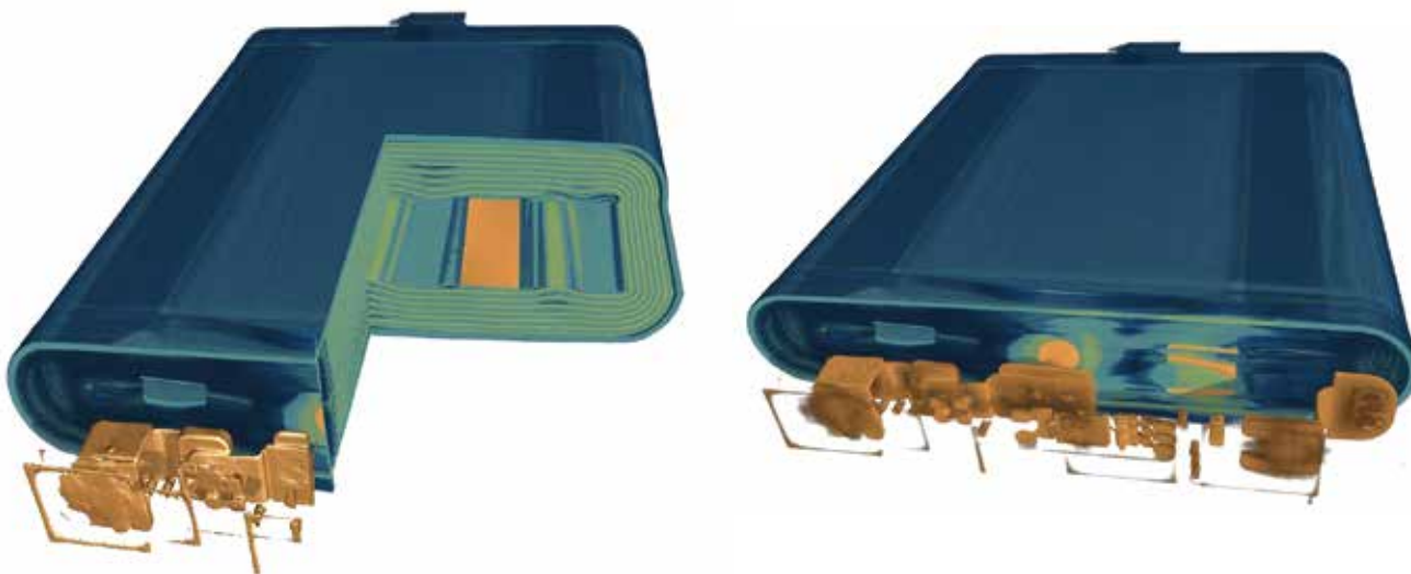
3D visualization of the volume obtained by X-Ray microtomography of a camera battery.
