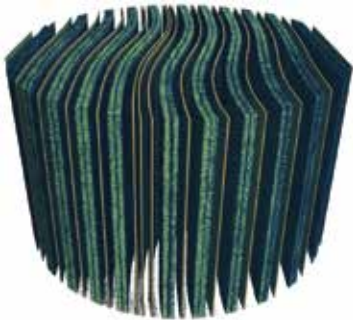
3D visualization of the internal layers of a battery, with highlighting of the phenomenon of electrode swelling.
