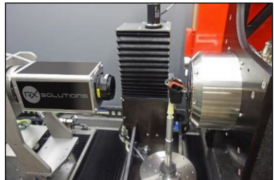
RX Solutions EasyTom 160 Multi-Purpose NanoTomograph
